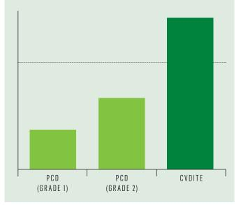
In applications where tool wear is dominated by abrasive wear CVD has been observed to show greater abrasion resistance compared to PCD. Therefore CVD is particularly suitable for highly abrasive continuous turning operations.
